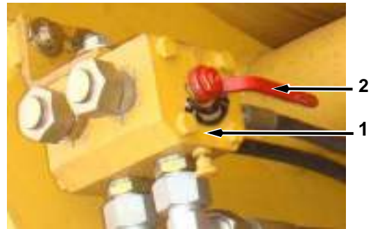
1. Diverter valve 2. Handle
